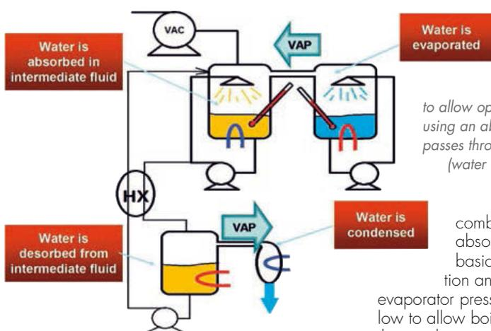
**Fig 1:** Working principle of pass-through distillation (PTD): the evaporation and condensation steps are decoupled to allow operation at different pressures, by using an absorption/desorption loop that passes through the component to be removed (water in this case)
