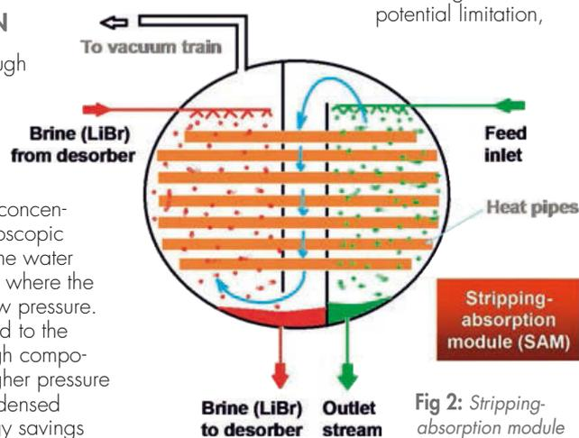
**Fig 2:** Stripping-absorption module (SAM) combining the evaporation and absorption steps into a single efficient unit (see [www.passthroughdistillation.com](http://www.passthroughdistillation.com) for detailed explanations)
